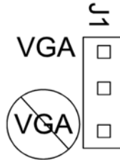
Figure 2: VGA Jumper Enlarged View
