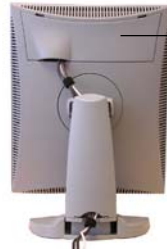
Signal cables routed under foot cover and bound by velcro strips
