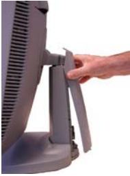
Push the upper side of the cover onto the foot
