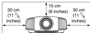
Air from air conditioners or the ventilation holes of this unit or other devices, may cause oscillation on the screen. Be sure not to install this unit in the area where the air from air conditioners or the ventilation holes of these devices reach to the front side of this unit.
