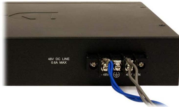
Figure 2- 4. Power connections attached to contacts after assembly
