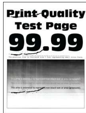
“Repeating defects” on page 417
